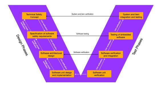
The ISO 26262 standard relies on the V-Model, which acts as a framework for matching requirements (left side) with corresponding tests (right side) to provide traceability.
