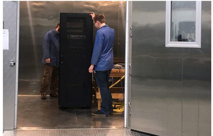
DC engineers preparing a rack enclosure for thermal performance testing
