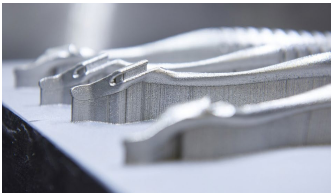
DanaMed's surgical tool before support removal and finishing.
