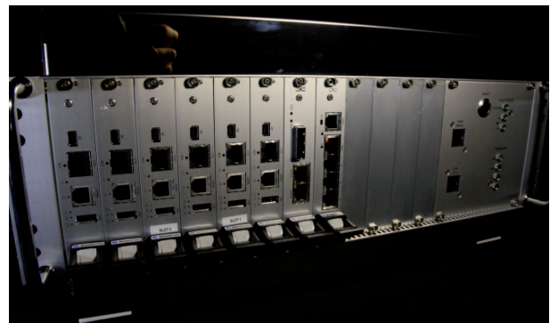
Figure 9a: StarVX parallel VPX computer, front view
