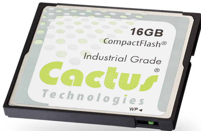
Figure 1. CompactFlash cards can be easily and quickly swapped for data logging systems and carrying out an update in the OS software.
