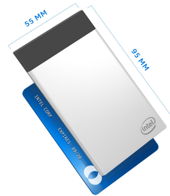
Figure 2. The Intel Compute Card is a credit-card sized modular computing platform (Source: Intel).
