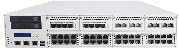
Figure 2. The PL-8120A is a 2U rackmount, high-performance solution for demanding NFV applications. (Source: WIN Enterprises)
