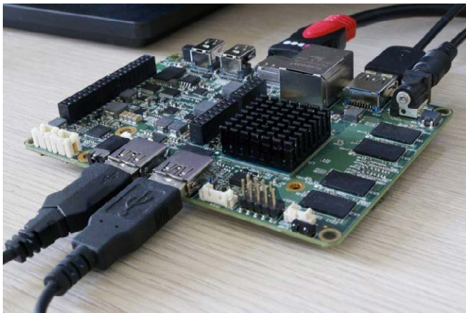
Figure 4. The UD00 x86 is an Arduino 101 development board. (Source: SECO)
