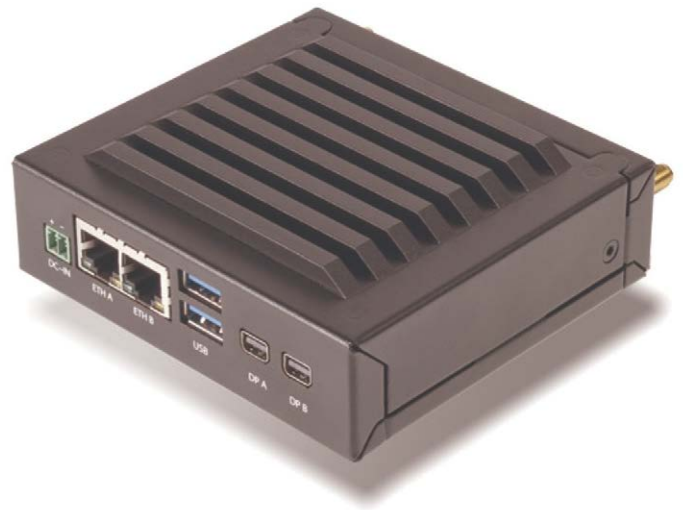
Figure 1. The MBox-V from TQ-Group supports flexible industrial firewalls. (Source: TQ-Group )
