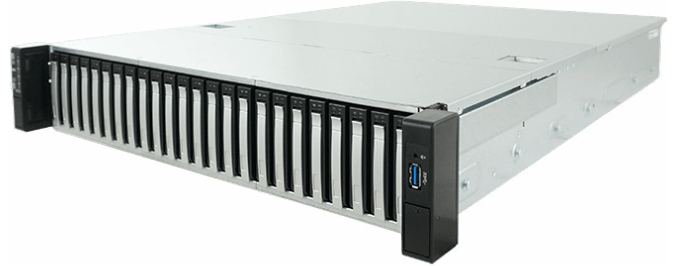
Figure 2. The FlacheSAN2N24U-D5 storage server from Premio Inc. uses the SSF to remove bottlenecks so it can reach to 60 Gbytes/s throughput, and 12 million IOPS. (Source: Premio Inc.)
