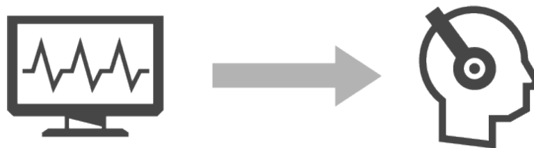
Figure 3. Experts can remotely listen for periodic phenomena because InsightCM can convert raw accelerometer data into a WAV file.
