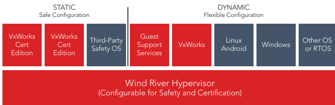
Figure 3. Static and dynamic configuration
