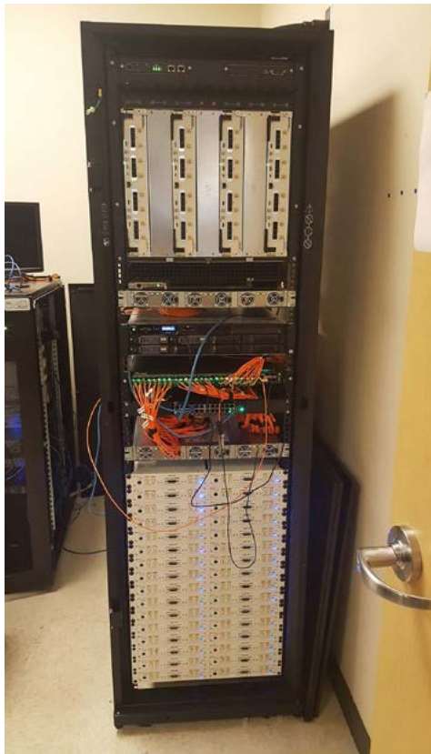
Figure 1. The DARPA Colosseum testbed features 128 Ettus X310 USRPs and NI ATCA-3671 processing units.
