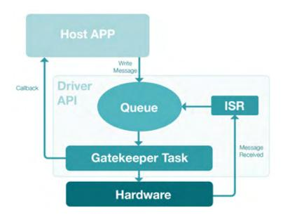
Figure 5. Architecture of a Gatekeeper Task
