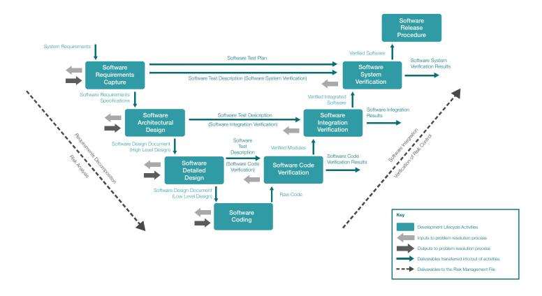
Figure 3. An example of an embedded software Safety Critical Development Lifecycle
