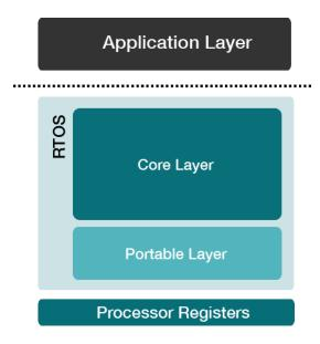
Figure 1. Typical internal structure of an RTOS
