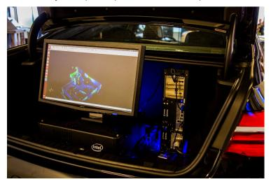
An autonomous vehicle is a complex piece of machinery encompassing wealth а of disparate electronic, electro-optic, and compute components and systems, including a combination of central processing units (CPUs), graphics processing units (GPUs), and field-programmable gate arrays (FPGAs), that must all work in tandem.
