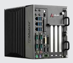
ADLINK's current flagship MXC-6400 Series of the Matrix line integrates a quad-core Intel® Core™ i7-6820EQ, which boasts a maximum Turbo Frequency of 3.5 GHz, while supporting silent, fanless operation. Industrial-friendly features include two front-mounted, hot-swappable SATA 3 Gb/s ports, a remote on/off power switch connected to
