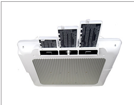
Figure 9. The integration of hot-swappable batteries makes the G series panel PCs highly suitable for mobile EMR applications.
