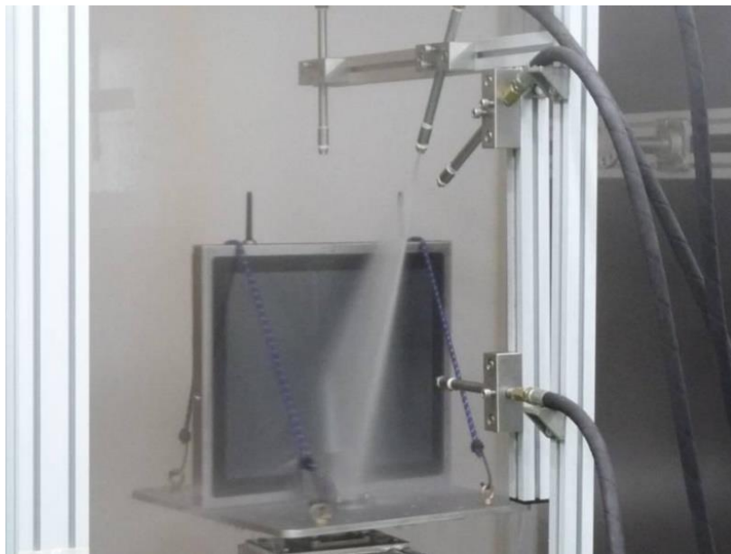
Figure 5. For guaranteed performance in harsh conditions, Wincomm subjects its box and panel PCs to a battery of tests using high-pressure water jets, LED leak lights, and vacuum pressure (Source: Wincomm).
