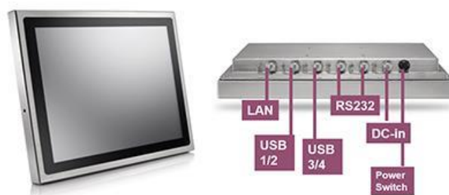
Figure 1. IP69K design expertise allowed Wincomm to develop a rugged HMI for an automated inspection system to be deployed in a harsh food and beverage factory environment (Source: Wincomm).
