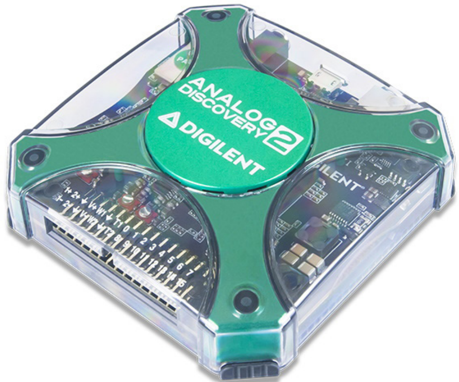
Figure 1. Analog Discovery 2 is a USB oscilloscope and multi-function instrument that allows users to measure, visualize, generate, record, and control mixed-signal circuits of all kinds. (Image source: Digilent)
