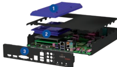
Figure 11: Depiction of the COM carrier system.
