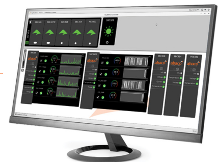
Figure 4: The HealthView GUI dashboard displays a summary on system components in the top section, with the lower section showing more detailed information for selected components.
