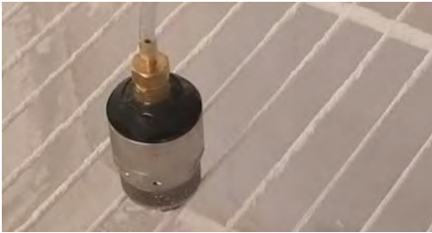
IP6X: Dust ingress test (under vacuum)—8hr with no incursion
